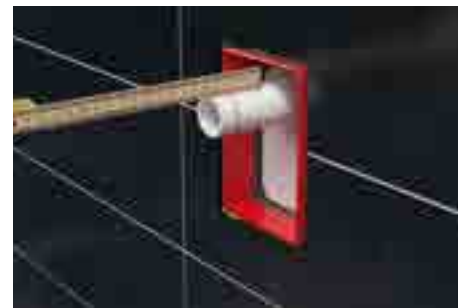
6. Mark 3cm, measured from the wall (tile)
