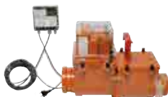
Typ 3: Anti-flooding valve with a self-acting closure, which is operated by external power (electric, pneumatic or others) and emergency closure, which is independent from the self-acting closure. HL710.2EPC, HL712.2EPC, HL715.2EPC
